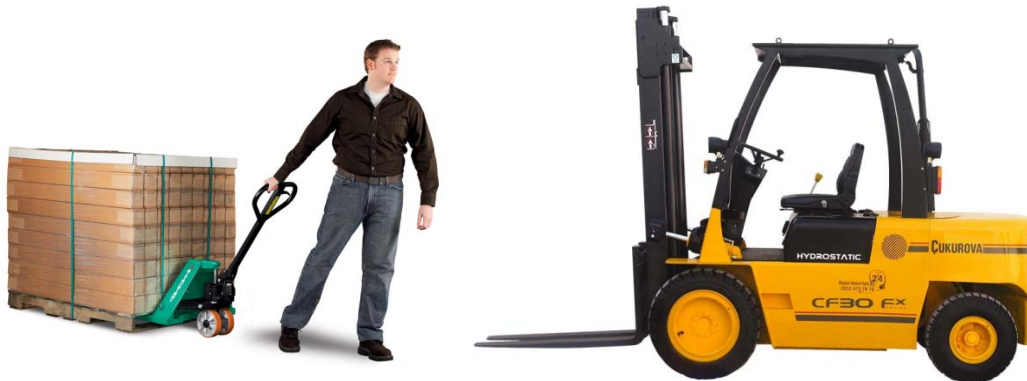
Picture 19. Forklift hand truck and forklift truck
