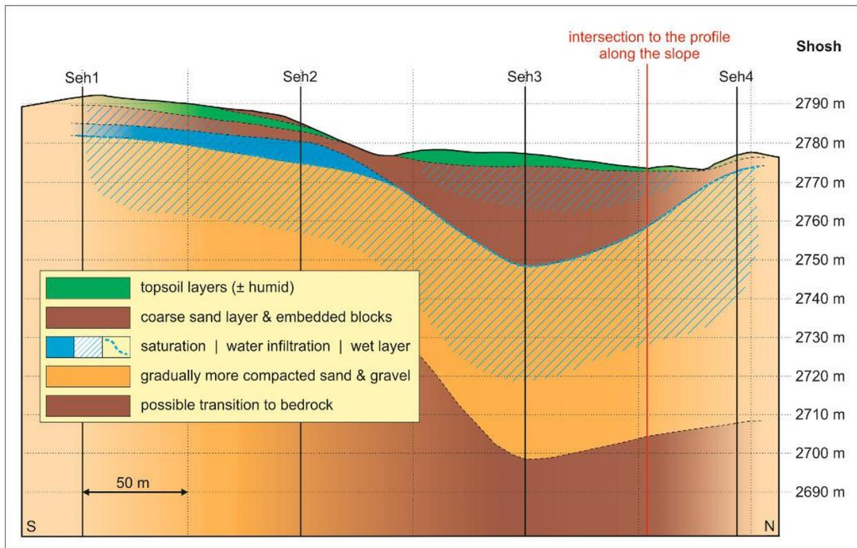
Fig. 9. Transversal cross-section (TCS) at Shosh. The dashed blue line refers to the main sliding surface identified by the geoelectrics survey. The second axis is stretched for better visualization.
