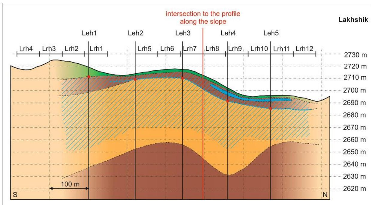
Fig. 10. Transversal cross-section (TCS) at Lakhshik. The red dots and the dashed blue line refer to the main sliding surface identified by both geophysical methods. The second axis is stretched for better visualization; colors are as indicated in Fig. 9.
