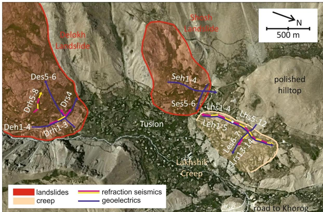
Fig. 4. Layouts of the refraction seismics and geoelectrics arrays in the three village parts (Google Earth, 2012).
