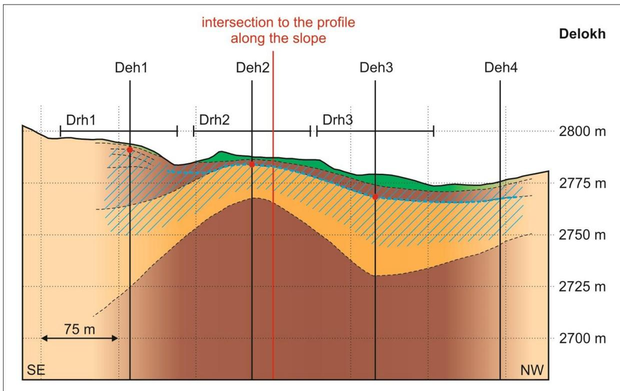
Fig. 6. Transversal cross-section (TCS) at Delokh. The red dots and the dashed blue line refer to the main sliding surface identified by both geophysical methods. The second axis is stretched for better visualization; colors are as indicated in Fig. 9.
